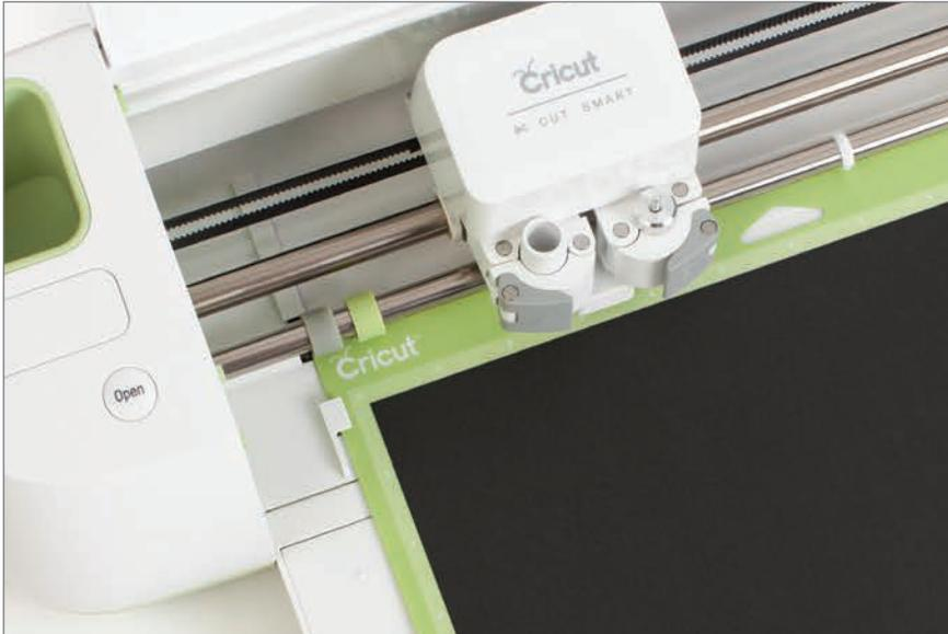
**Tip:** You will know the mat is loaded correctly when the Cricut logo on the mat is directly under the machine rollers.
