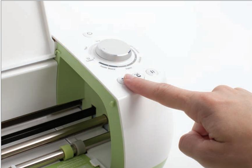
**Tip:** Be sure to remove your pen—just open accessory clamp A and pull the pen straight up. Don't forget to cap the pen!
