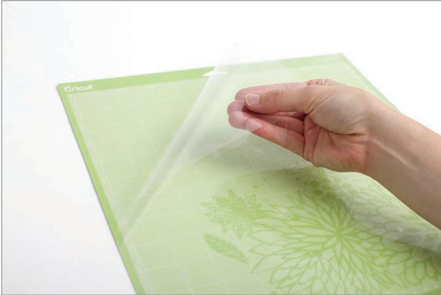
**Tip:** Set this cover aside while you cut but be sure to replace to protect the mat's adhesive during the times it is not in use.
